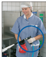
8. Turn on the water tap and start the foam application by pressing the "trigger".
