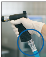
7. The hose with 1/2" quick-coupling is connected to nipple on the water gun.
