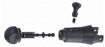
Remove the Percussion Hammer (part °903) with spring (part °904) and then Percussion Trigger (part °902) with spring (part °905) will come out by themselves.
