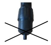
Arm the system and press on the percussion trigger (the gun must always be pointed downwards, even if it's not loaded!). You must feel the movement of the percussion hammer (part °903).
