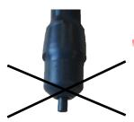
Check that the punching pin is retracted in the barrel
