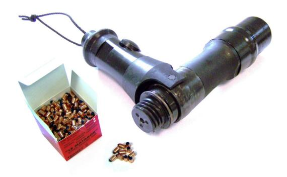
When the trigger is pushed, explosion of the cartridge generates gas that pushes the pin at 50m/s (180km/h). The MATADOR is in contact with the head of the animal and the pin will penetrate the brain. The animal is immediately anesthetized and must be bled as soon as possible.
