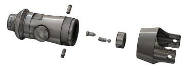
When changing the Ejection Base holder 907B by a new one, there is chances that both holes on parts 907B and Safety Grip 901B will not be in line. Then Pins 908
