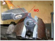
Remove the 2 Holding Pins 908. Use a Screw Driver to help removing Pins 908. The Ejection Base Holder 907B and the Firing Pin 906 can then be removed.
